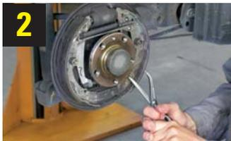
2 Always use an appropriate special tool for fitting / removing the **return springs**
