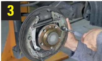
3 To prevent damage to the components, always use appropriate special tool for fitting / removing the **retaining spring**
