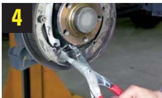
4 To prevent damage to the components, always use appropriate special tool for fitting / removing the **hand brake cable**
