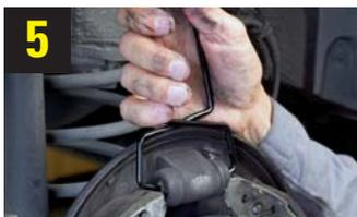
5 When removing the brake shoes, secure the brake pistons with appropriate tools.
