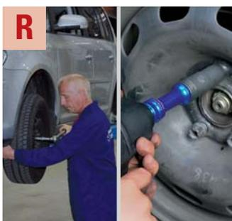
R To prevent wheel hub damage and / or lateral run-out of the brake discs, the wheel bolt / nut must be tightened according to the manufacturer's specifications (sequence + torque).
