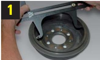
1 Check brake drum for wear and damage. Measure diameter. New dimension plus 0.5 mm max. diameter can only be used with over-sized drum brake linings. Depending on the version, wheel bearings and/or sensor rings are also replaced.
